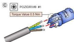
**C** Insert the wire into the terminals and fasten the clamping device with a POZIDRIV® #1, max. Torque 0.5 Nm (0.37 lb-ft).
